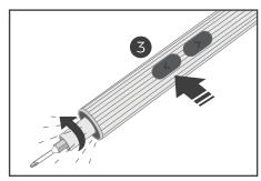
2. Press 3, Tighten the screw and turn on the light at the same time.
