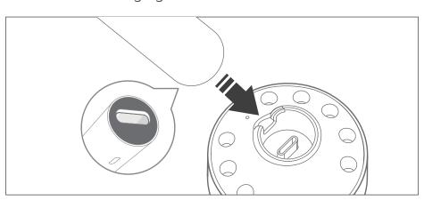
6. When charging, align the end connector of the electric screwdriver with the charging port of the charging base, the light on the end of the electric screwdriver means charging.
