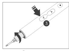
2. Press 3, tighten the screws.
