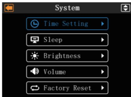
**Brightness setting:** Click the progress bar or long press the left or right key to adjust the brightness.
